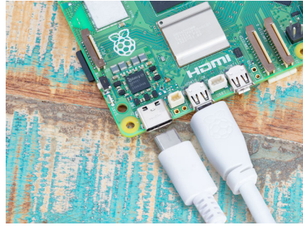
Figure 2-18 Powering your Raspberry Pi 5
